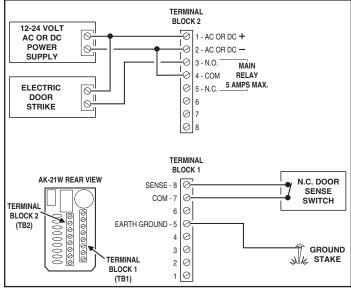
Figure 8. Basic Door Installation Wiring
